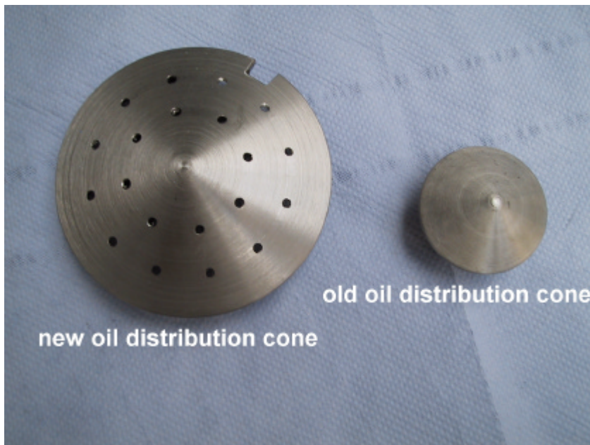
Figure 4: New and conventional design conception of the compressor distribution cone [3]
